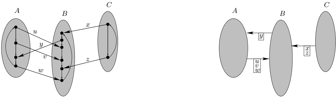
Figure 1: The time-expanded graph (left) and the time-dependent graph (right) of a timetable with three stations A, B, C. There are three trains that connect A with B (elementary connections u, v, w ), one train from C via B to A ( x, y ) and one train from C to B ( z ).
