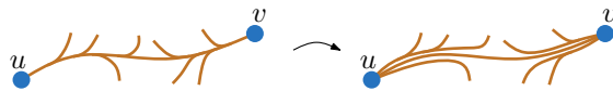
Fig. 4. Any strict confluent drawing of a graph without a K_{2,2} subgraph can be transformed into a standard planar drawing.
