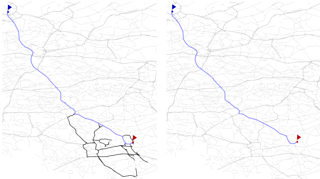
Figure 4.3: Search space of a typical uni-(left) and bidirectional(right) SHARC-query. The source of the query is the upper flag, the target the lower one. Relaxed edges are drawn in black. The shortest path is drawn thicker. Note that the bidirectional query only relaxes shortest-path edges.
