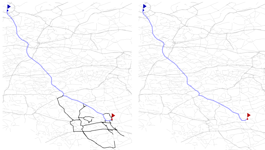
Fig. 1. Search space of a typical uni-(left) and bidirectional(right) SHARC-query. The source of the query is the upper flag, the target the lower one. Relaxed edges are drawn in black. The shortest path is drawn thicker. Note that the bidirectional query only relaxes shortest-path edges.
