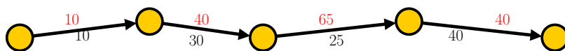
Fig. 3.11: Reach values of a sample path. Black numbers represent edge lengths, red numbers reach values.
