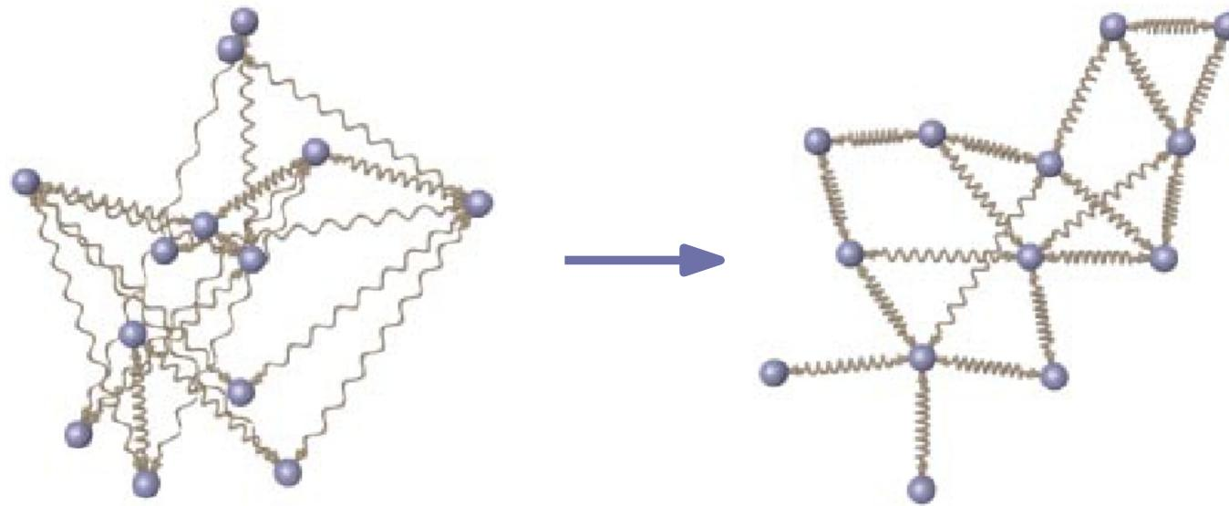
“To embed a graph we replace the vertices by steel rings and replace each edge with a spring to form a mechanical system . . . The vertices are placed in some initial layout and let go so that the spring forces on the rings move the system to a minimal energy state.” [Eades, '84]
