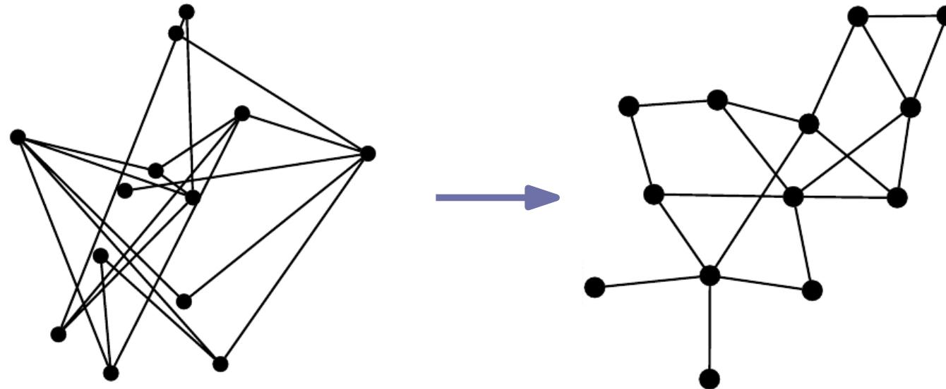
So-called **spring-embedder** algorithms that work according to this or similar principles are among the most frequently used graph-drawing methods in practice.
