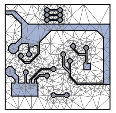
To simulate the heat produced on boards we can use the *finite element method* (FEM):
