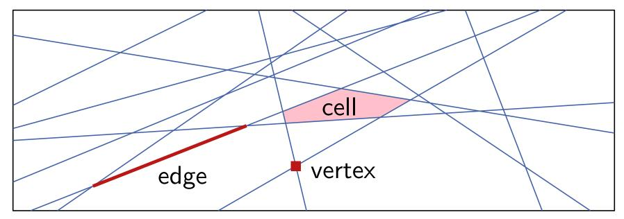
**Def:** A set L of lines defines a subdivision  $\mathcal{A}(L)$  of the plane (the **line arrangement**) composed of vertices, edges, and cells (poss. unbounded).
