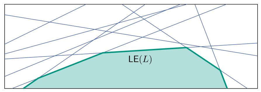
**Def:** For a set L of lines the **lower envelope** LE(L) of L is the set of all points in  $\bigcup_{\ell \in L} \ell$  that are not above any line in the set L (boundary of the intersection of all lower halfplanes).
