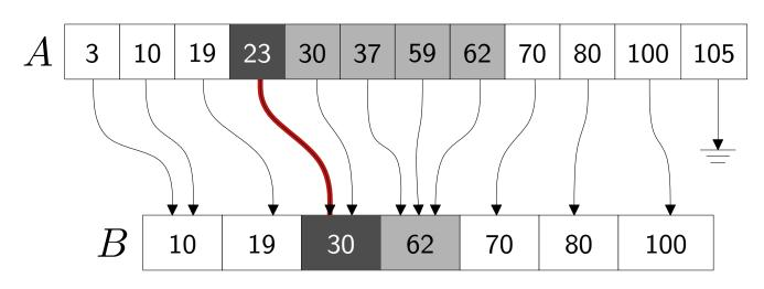
link  $a \in A$  with smallest  $b \ge a$  in B
