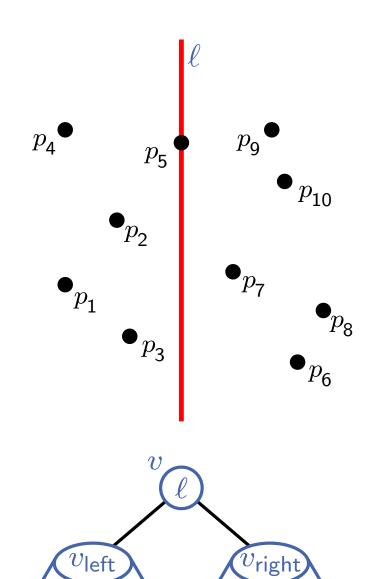
$\begin{aligned} & \textbf{BuildKdTree}(P, depth) \\ & \textbf{if } |P| = 1 \textbf{ then} \\ & | \textbf{ return leaf with a point in } P \\ & \textbf{else} \\ & | \textbf{ if } depth \textbf{ even then} \end{aligned}$
