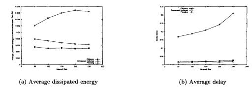
Figure 4: Directed diffusion compared to flooding and omniscient multicast.
