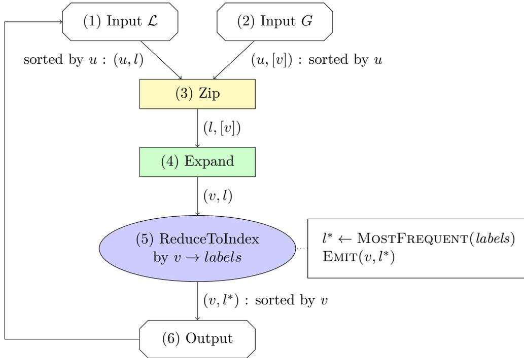
Figure 3.2: Distributed Label Propagation
