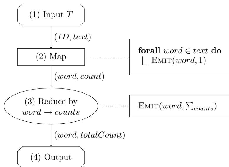
Figure 3.1: The Word Count Algorithm in MapReduce
