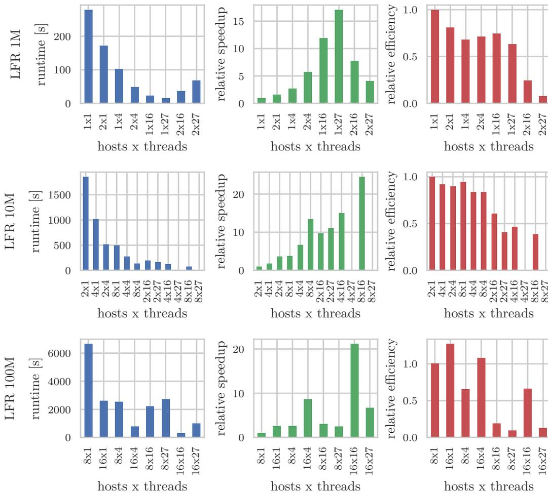
Figure 4.2: Label propagation scaling for three LFR graphs with different host and thread per host configurations. The configurations are ordered by the total thread count. Speedup and efficiency are calculated in relation to the configuration with the fewest total threads.
