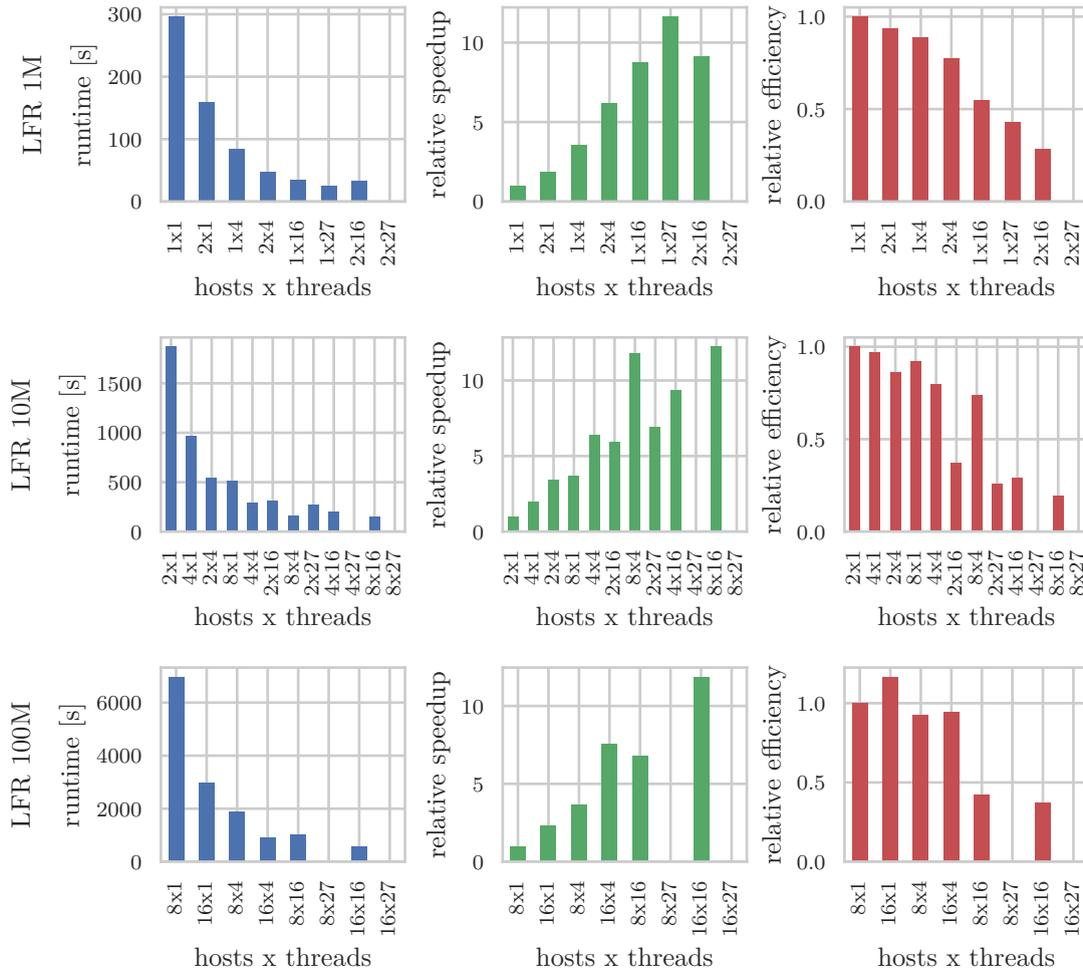
Figure 4.5: DLSLM scaling for three different types of graphs with different host and thread per host configurations. The configurations are ordered by the total thread count. Speedup and efficiency are calculated in relation to the configuration with the fewest total threads.
