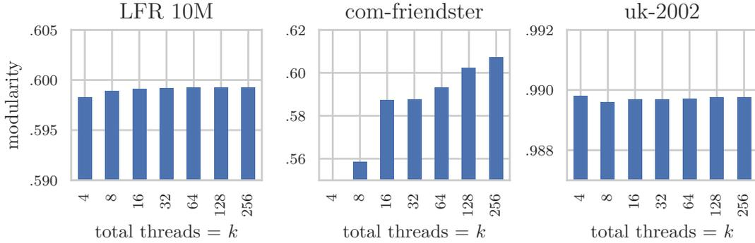
Figure 4.4: DLPLM modularity results for different total thread counts and thus partition sizes  $k$ .
