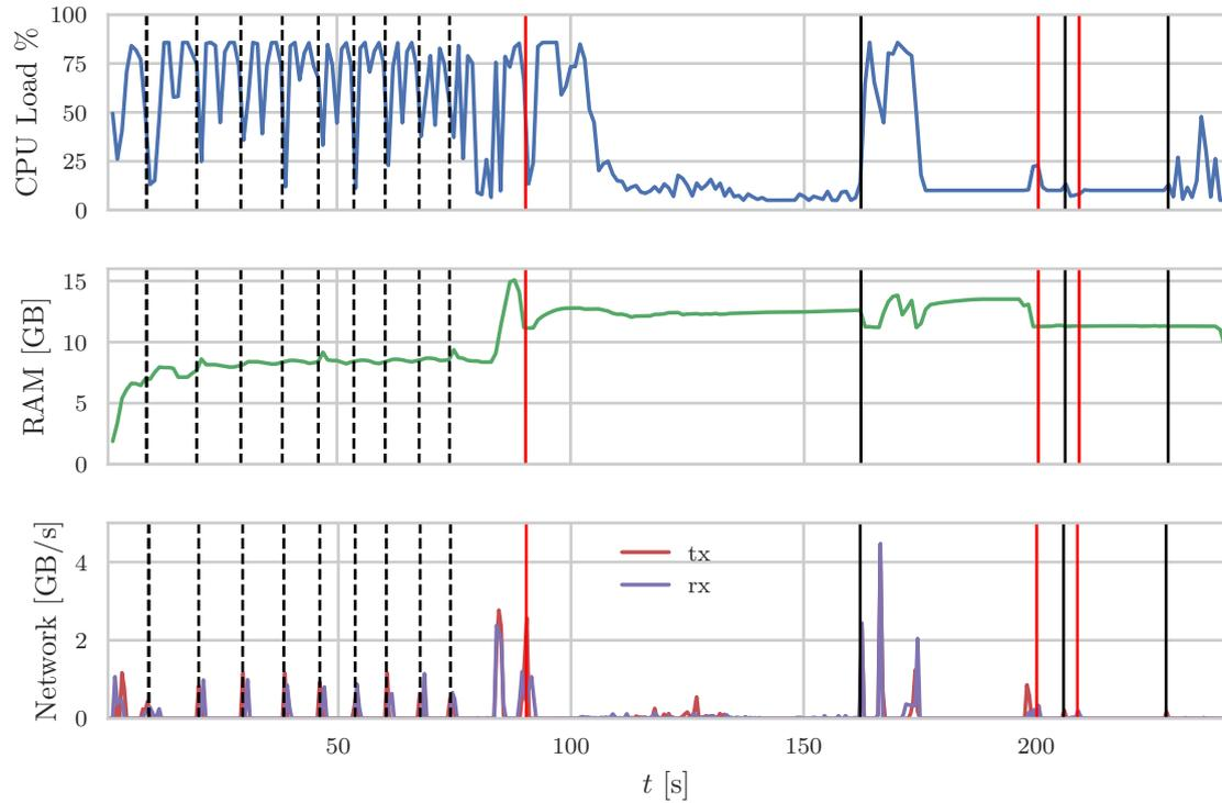
Figure 4.6: Resource usage on one of eight hosts performing DLPLM on LFR 10M. Dashed lines indicate the start of a label propagation iteration, but only on the first level. Red lines mark the start of the partitioned local moving. The continuous black lines indicate the contraction phase.
