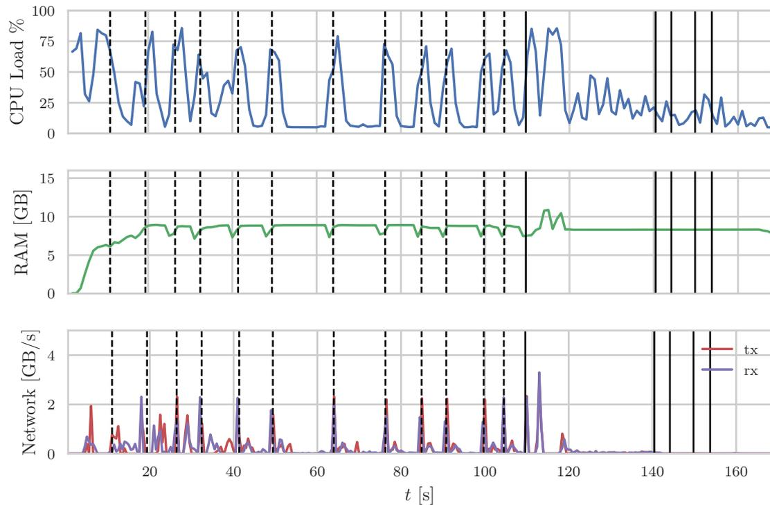
Figure 4.7: Resource usage on one of eight hosts performing DLSLM on LFR 10M. Dashed lines indicate the start of a synchronous local moving iteration, but only on the first level. The continuous lines indicate the contraction phase.
