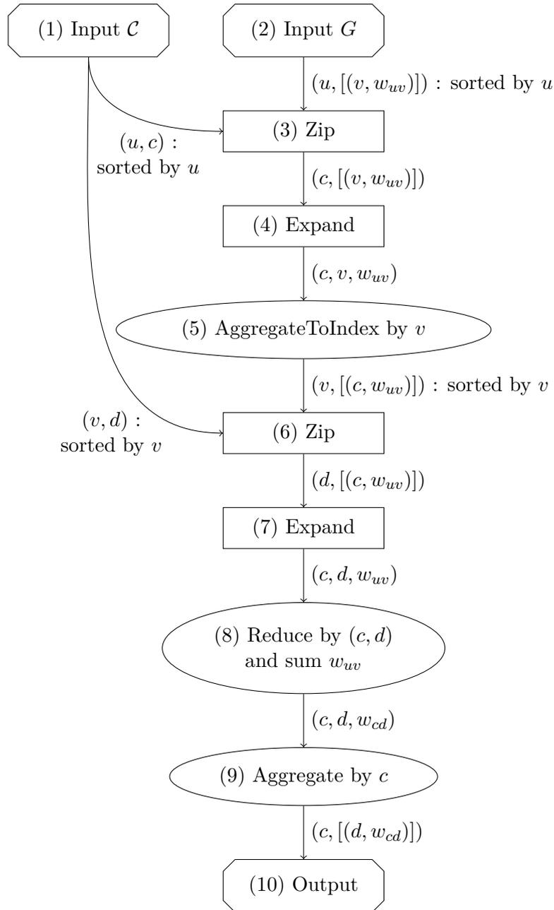
Figure 3.7: Distributed Contraction without Joins
