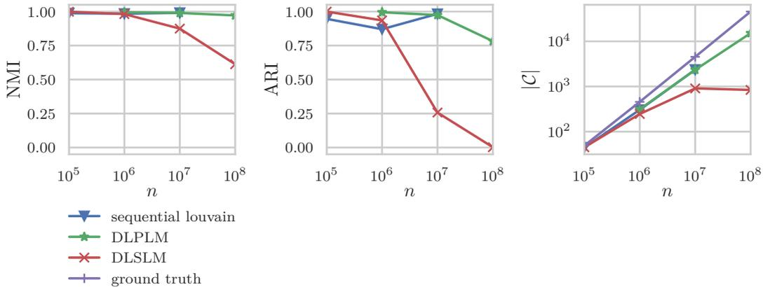
Figure 4.9: Similarity of clustering results to ground truth of our LFR graphs by graph size and algorithm. The third chart shows the number of clusters in the clustering retrieved by each method.
