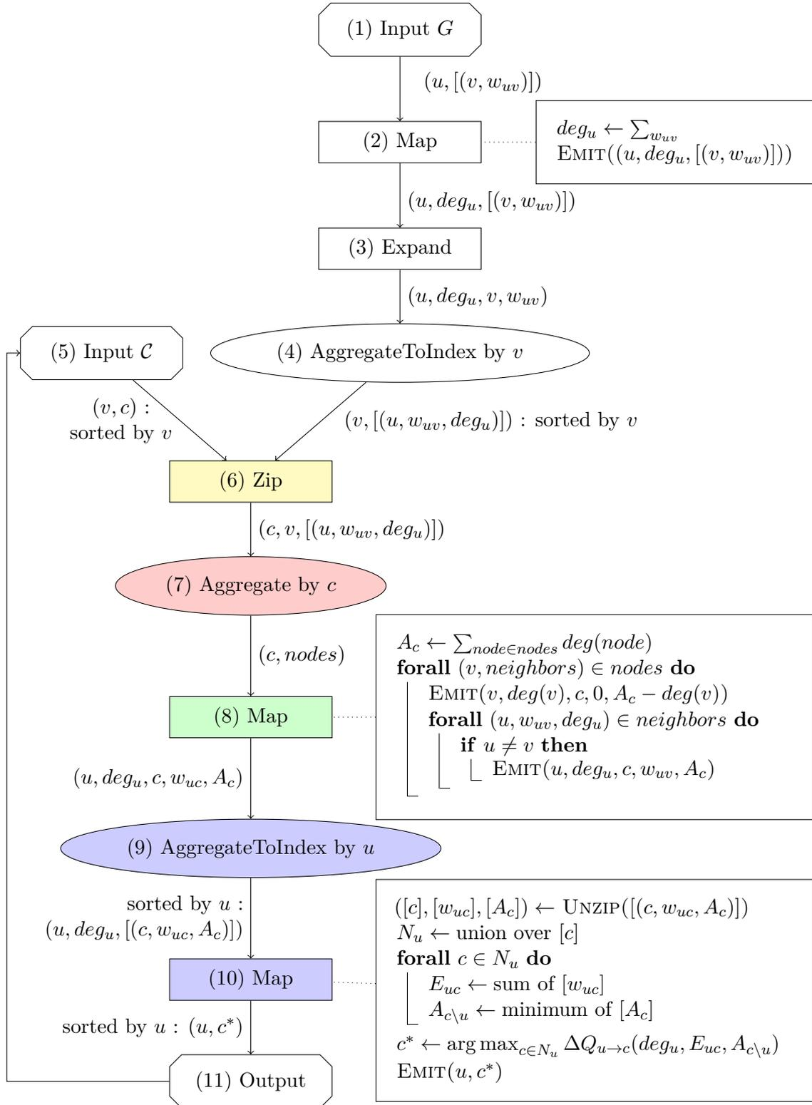
Figure 3.5: Synchronous Local Moving
