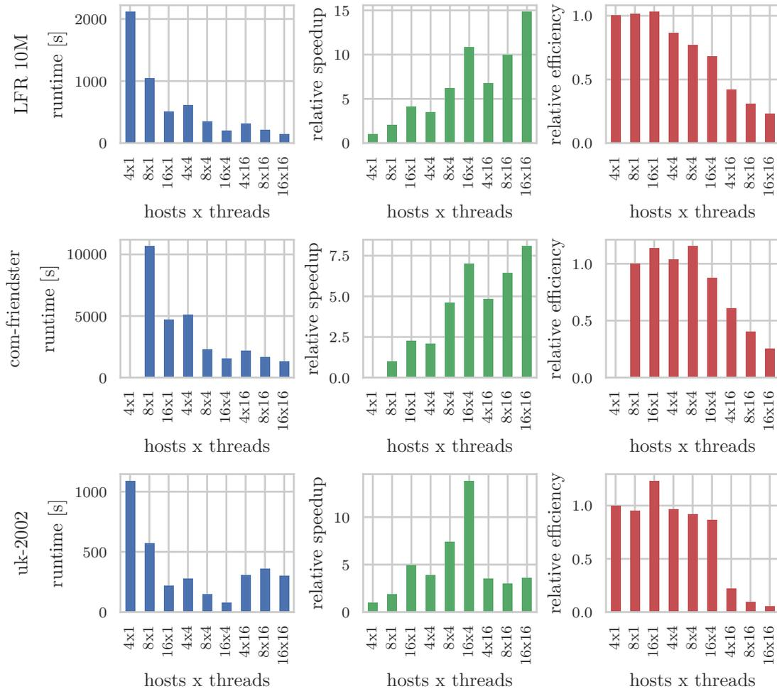
Figure 4.3: DLPLM scaling for three different types of graphs with different host and thread per host configurations. The configurations are ordered by the total thread count. Speedup and efficiency are calculated in relation to the configuration with the fewest total threads.
