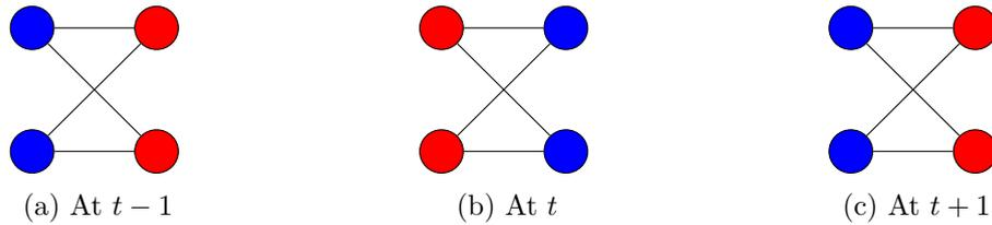
Figure 2.2: Example of label oscillation in a bipartite graph
