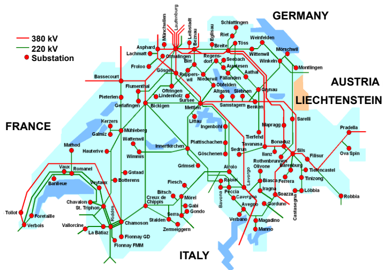
Figure 4.1.: Transmission network of Switzerland from [3].
