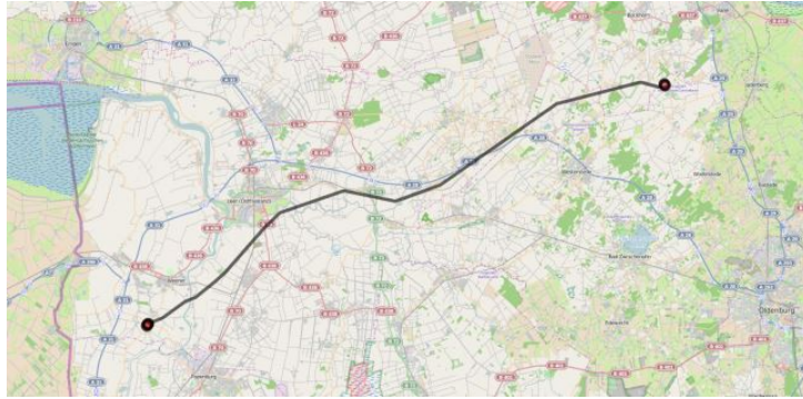
Figure 4.5: Example of a relation constituted of two substations. The two red circles are the two substations contained in the relation (OSM-ID=1637161) and the black line are the transmission lines (this relation contains four transmission lines)[Med18].
