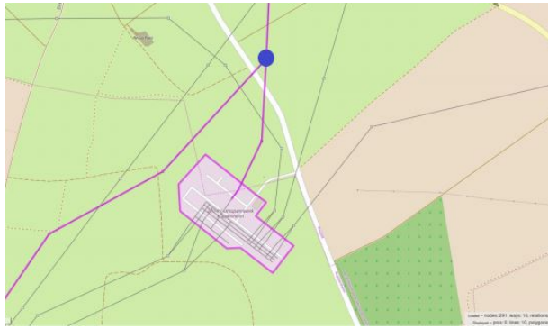
Figure 4.7: T-connection from relation (OSM-ID=339244). The T-node represented by the blue filled circle, is the node at which the transmission line at the top part of the figure branch into two parts. Figure obtained using overpass-turbo.eu, credits: ©OpenStreetMap contributors[Med18].
