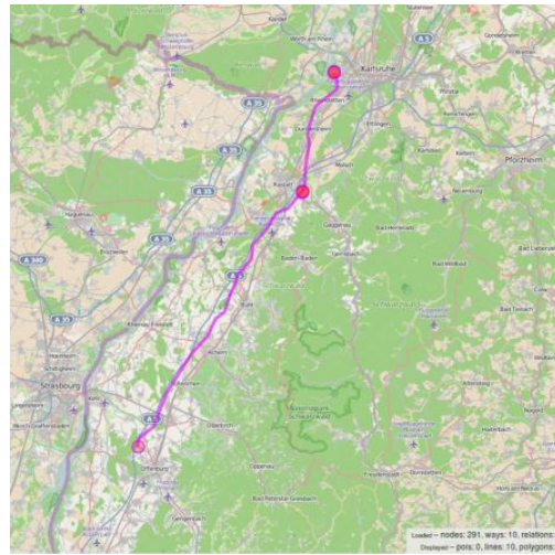
Figure 4.6: Example of a relation (OSM-ID=339244) containing three substations (circles), a T-junction and seven transmission lines. Figure obtained using overpass-turbo.eu, credits: ©OpenStreetMap contributors[Med18].
