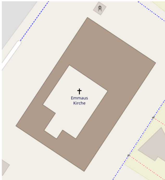
Figure 4.1: A church presented in OSM, which consists of one outer and one inner ring. ((OSM-ID=1596371))
