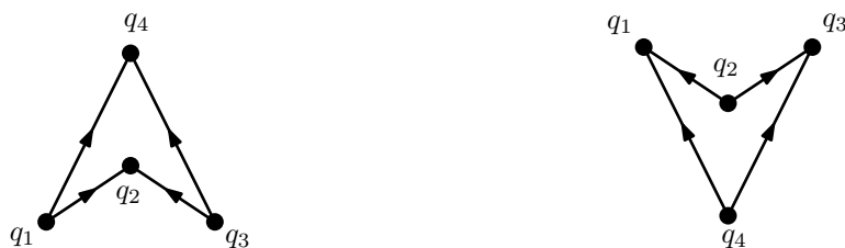
Figure 5.13: The two base cases for constructing a nice upward planar quasi-4-tree G with only global sources and global sinks.
