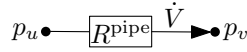
Figure 5.4: Model of a hydraulic pipeline which connects two vertices u and v , where there is a pressure p_u or p_v , respectively. The resistance of the pipeline is denoted by R^{\text{pipe}} and the flow by \dot{V} . The resistance for gas network lines is R^{\text{pipe}} = R^g and for heat network lines R^{\text{pipe}} = R^h .
