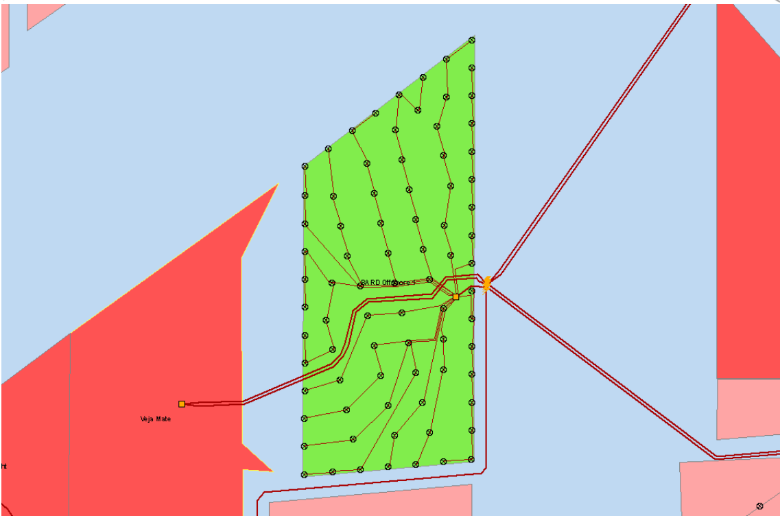
Figure 1.2: Screenshots from the Global Offshore Wind Farm Map by 4C Offshore [4coc], showing the BARD Offshore 1 Wind Farm. The nearby red shaded wind farms are projects under construction, and the pink ones are being planned (as of May 2016). The first map shows the north of German and the North Sea. The second image is a zoomed-in view of BARD Offshore 1. We see its turbines, its own substation, the near BorWin 1 converter station as well as cables interconnecting the sites.
