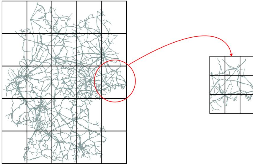
Figure 4: Illustration of a two-level partition. The first-level is a  $5 \times 5$  grid and each coarse region is partitioned in the second-level by a  $3 \times 3$  grid. For each edge, the bit-vector for the coarse grid and the bit-vector for the fine grid *in the same region as the edge* is stored.
