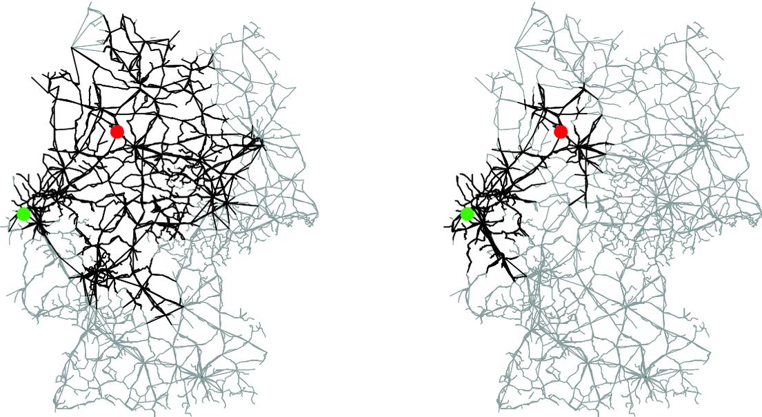
Figure 5: Reduction of the search space by using a bidirectional search (the search space of a standard DIJKSTRA search is shown on the left. The right figure illustrates the search space of a bidirectional search.).
