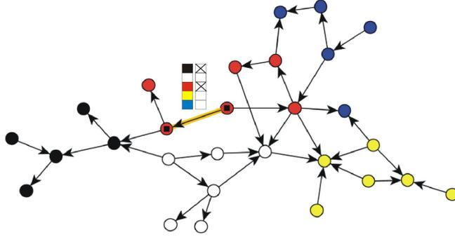
Figure 3: Illustration of the partition-based acceleration: the marked edge only leads to red and black nodes. A search with targets in blue, yellow or white regions can ignore this edge.
