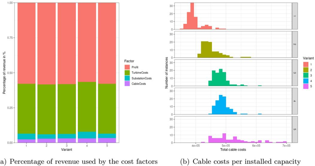
Figure 5.6: This figure provides an overview of the costs of the MILP solutions. For each variant, the left figure 5.6(a) shows what percentage of the revenue is used for profit, substation costs, turbine costs, and cable costs. For each instance and variant, the right figure 5.6(b) shows the ratio cable costs per installed capacity.
