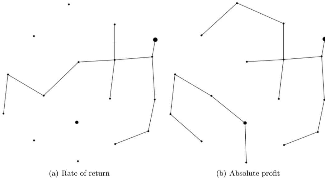
Figure 5.1: This figure shows the flow graph calculated by the MILP with objective maximize rate of return (see 5.1(a)) and with the objective maximize the absolute profit (see 5.1(b)). If we maximize the rate of return, only one substation is chosen. The more suitable solution is calculated if the objective is to maximize the absolute profit.
