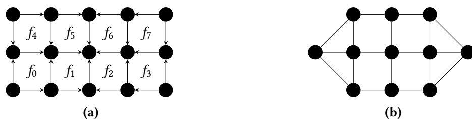
Figure 3.30: On the left, the Cartesian product of Figure 3.29 as a grid. On the right, the 3-connected graph we get by substituting the vertices with degree 2 with an edge.
