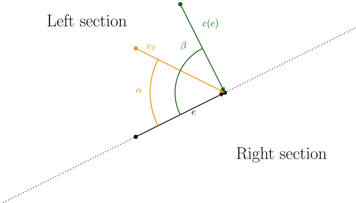
Figure 5.4: The idea behind the formula Embedding. Here, the embedding is not fulfilled as  $\cos(\beta) > \cos(\alpha)$  and thus  $\alpha < \beta$ .
