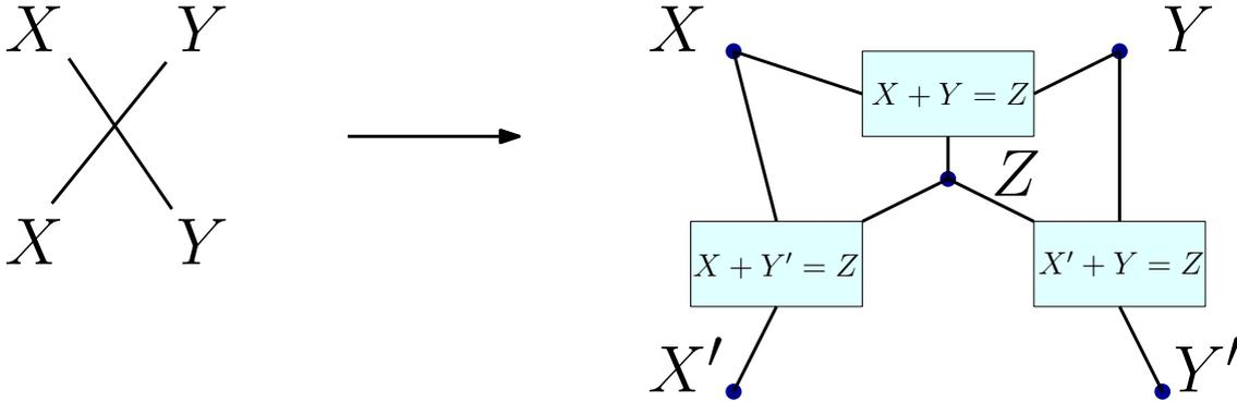
Figure 3.1: Crossing Gadget for PLANAR-ETR-INV (Original: [DKMR18])
