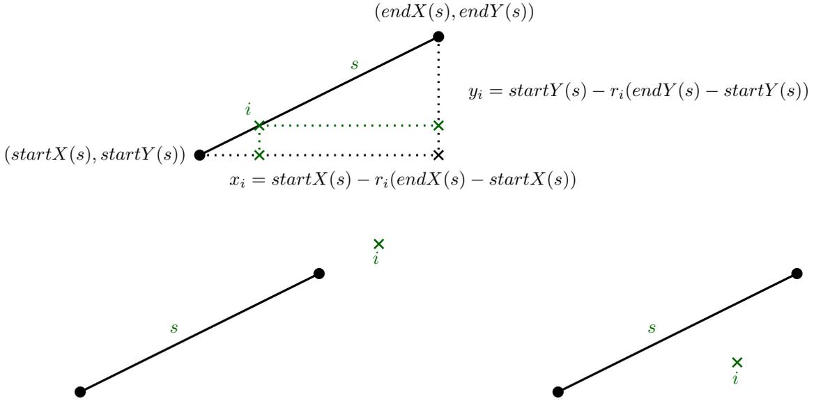
Figure 5.2: Visualization of the idea behind the formula  $\text{OnSegment}$ . Top:  $r_i$  exists and is between 0 and 1, bottom left:  $r_i$  exists, but is greater than 1, bottom right:  $r_i$  does not exist
