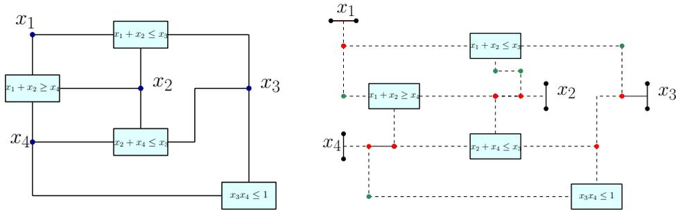
Figure 5.13: Reduction from the planar incidence graph to DRAWINGONSEGMENTS. The red dots represent split gadgets, the green ones represent turn gadgets. The dashed lines are implemented with copy gadgets. (Original: [LMM18])
