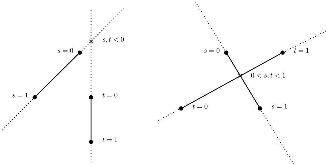
Figure 5.3: Visualization of the idea behind the formula LineIntersection
