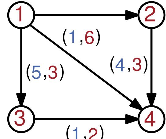
Algorithm B. (Denote by  $g_j(c)$  the time of the quickest 1-j t-path with length is at most  $c$ )
