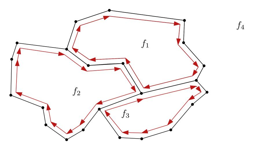
For each edge of internal faces introduce directed half-edge (clockwise)
