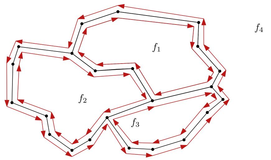
For each edge of internal faces introduce directed half-edge (clockwise) For each edge of external face introduce directed half-edge (counter-clockw.)
