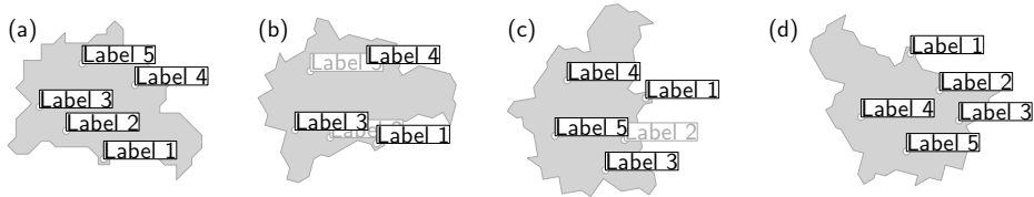
Fig. 1: Input map with five points (a) and three rotated views with some partially occluded labels (b)–(d).
